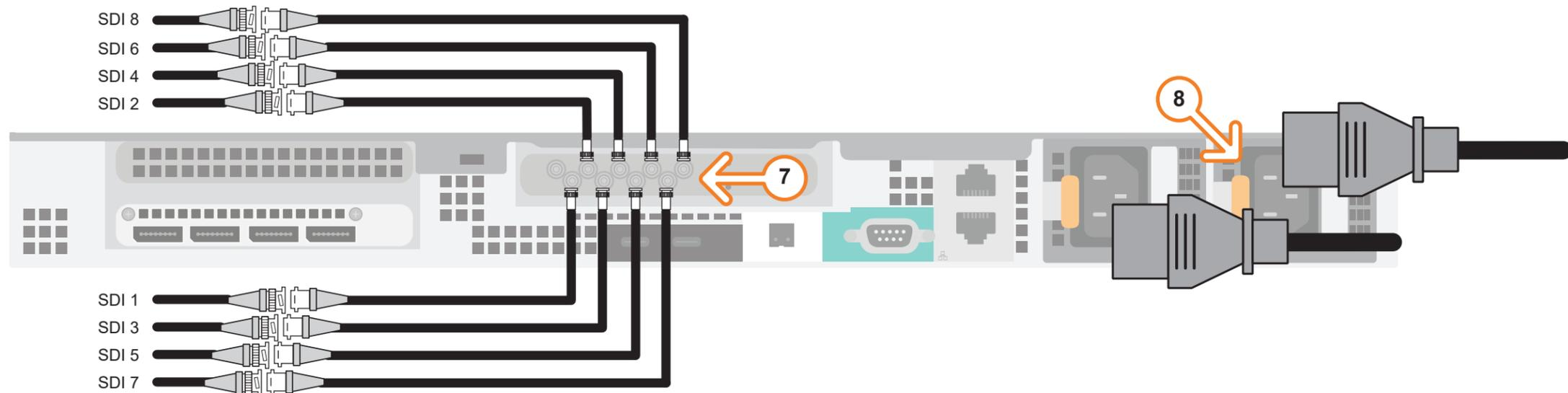
**7** Connect the HD-BNC end of the pigtail cables to the HD-BNC connectors and attach the SDI cables to the BNC end of the pigtails according to their required destination (see the *XPression User Guide* or Help file for information about configuring the key and fill for the HD-BNC connectors). The default configuration is displayed in the table below.
